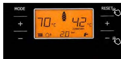
Figure 9 Ending the deaeration function
